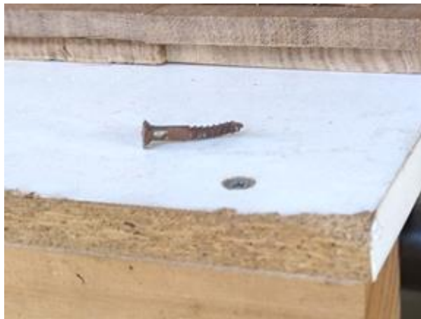
Screw found in thickness planer
